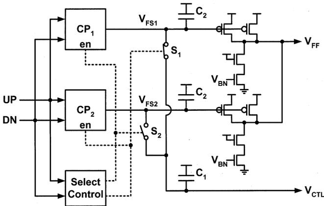
Fig. 6. Sampled feedforward circuits.
