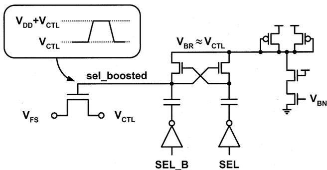
Fig. 7. Feedforward network bias switches.
