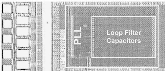
Fig. 13. Die micrograph of the self-biased clock generator PLL.
