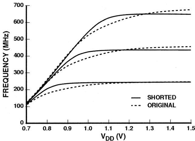
Fig. 12. VCO frequency as a function of supply voltage for three control voltages before shorting (dashed line) and after shorting (solid line) differential pair tail nodes.
