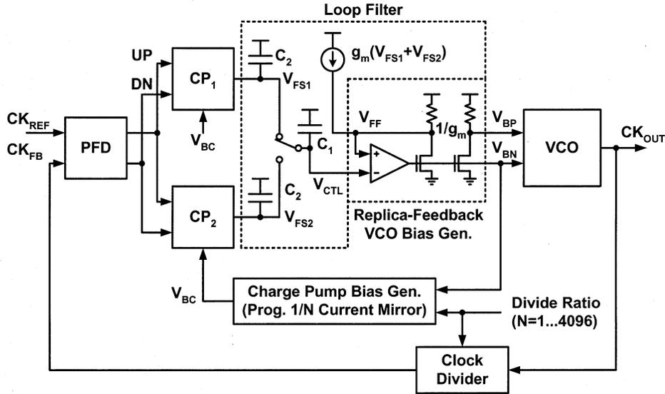
Fig. 5. Self-biased clock generator PLL architecture.
