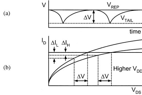
Fig. 10. Differential pair (a) tail node voltages and (b) tail currents as a function of time.
