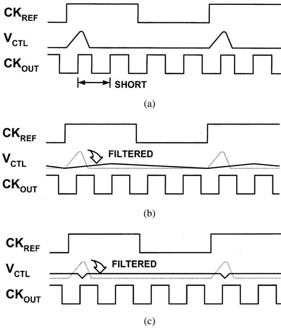
Fig. 3. Pattern jitter on output clocks with (a) simple second-order PLL, (b) added shunt capacitor, and (c) sampled feedforward network.
