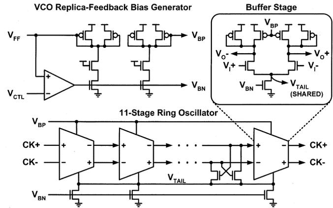
Fig. 11. Modified VCO circuits with shorted differential pair tail nodes.
