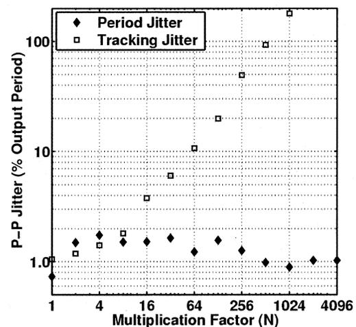
Fig. 14. Jitter versus multiplication factor at fixed 240-MHz output.
