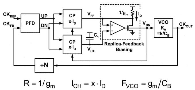
$$R = 1/g_m \quad I_{CH} = x \cdot I_D \quad F_{VCO} = g_m/C_B$$
