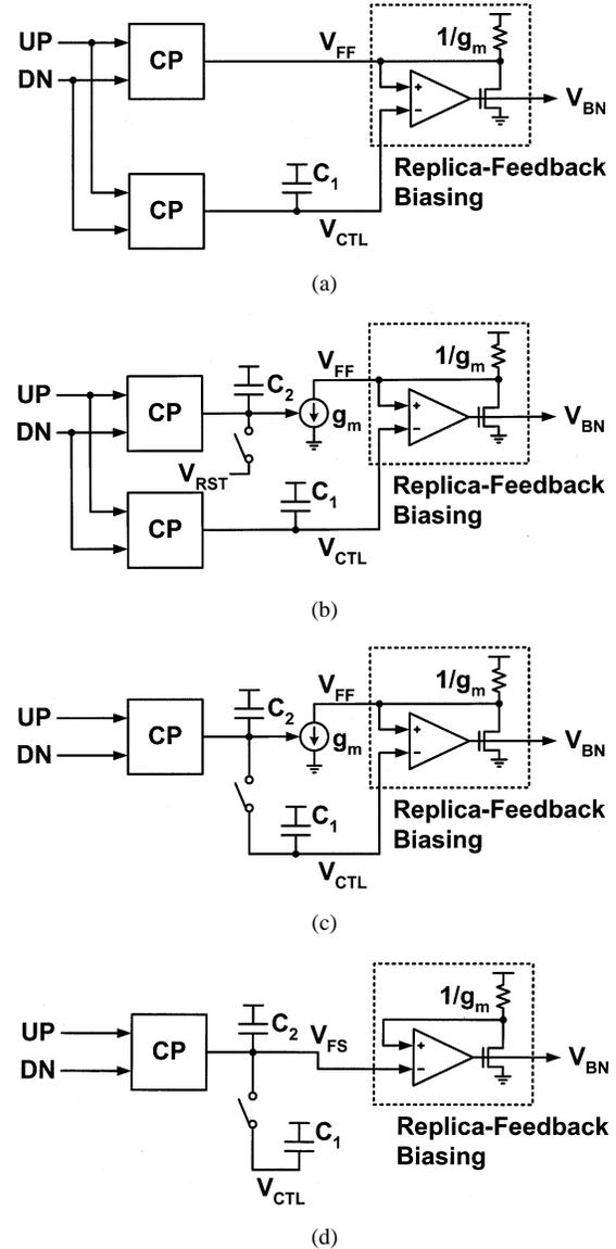
Fig. 4. PLL loop filter network (a) for simple self-biased PLL, (b) with sampled feedforward network, (c) with sampled feedforward network with  $C_2$  reset to  $C_1$ , and (d) with sampled feedforward network with  $C_2$  driven directly into amplifier.
